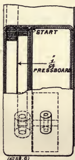
Figs. 242 and 243.—Field Winding, 35 Horse-power Johnson-Lundell Motor.
